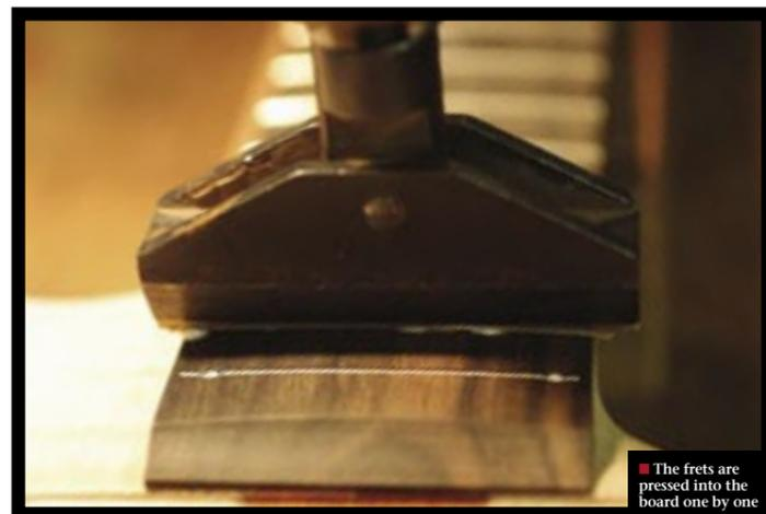
The frets are pressed into the board one by one
