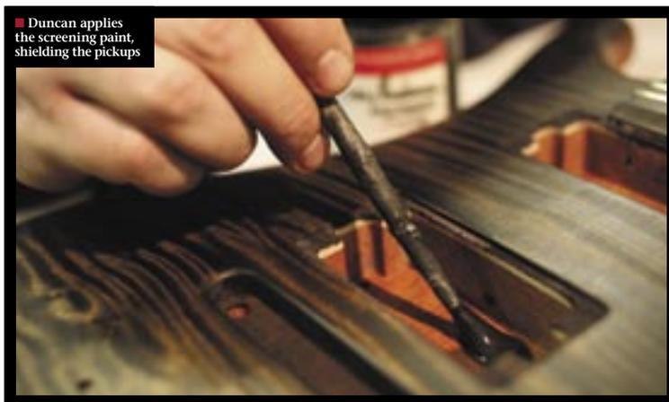
■ Duncan applies the screening paint, shielding the pickups
