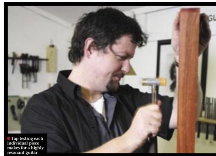
Tap testing each individual piece makes for a highly resonant guitar
